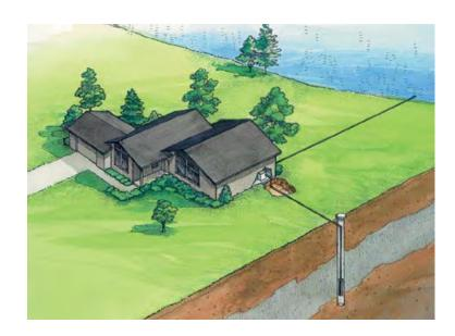
Open-loop systems use groundwater from a well as a heat source.
